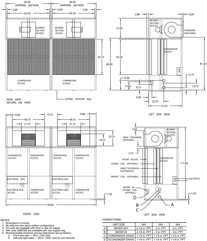
С CONDENSATE DRAIN 1-1/4 in. FPT 1-1/4 in. FPT 1-1/4 in. FPT ECONOMIZER DRAIN 1-1/4 in. FPT 1-1/4 in. FPT D 1-1/4 in. FPT REPLACEMENT FILTERS : SIXTEEN (16) AT 17 x 27 x 4 INCHES.
